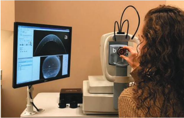
FIGURE 3. RTVue OCT (Optovue, Fremont, CA) as set up in an eye bank. A, Customized software is designed for analyzing corneal tissue in preservation medium. B, An adaptor for cornea viewing chambers makes tissue positioning easy. The operator makes fine adjustments and then can lock the chamber in place with an adjustment screw.
